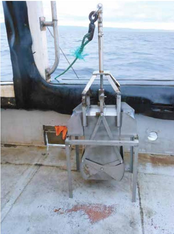
Figure 5.1. The box core used to retrieve sediment from the seafloor.
