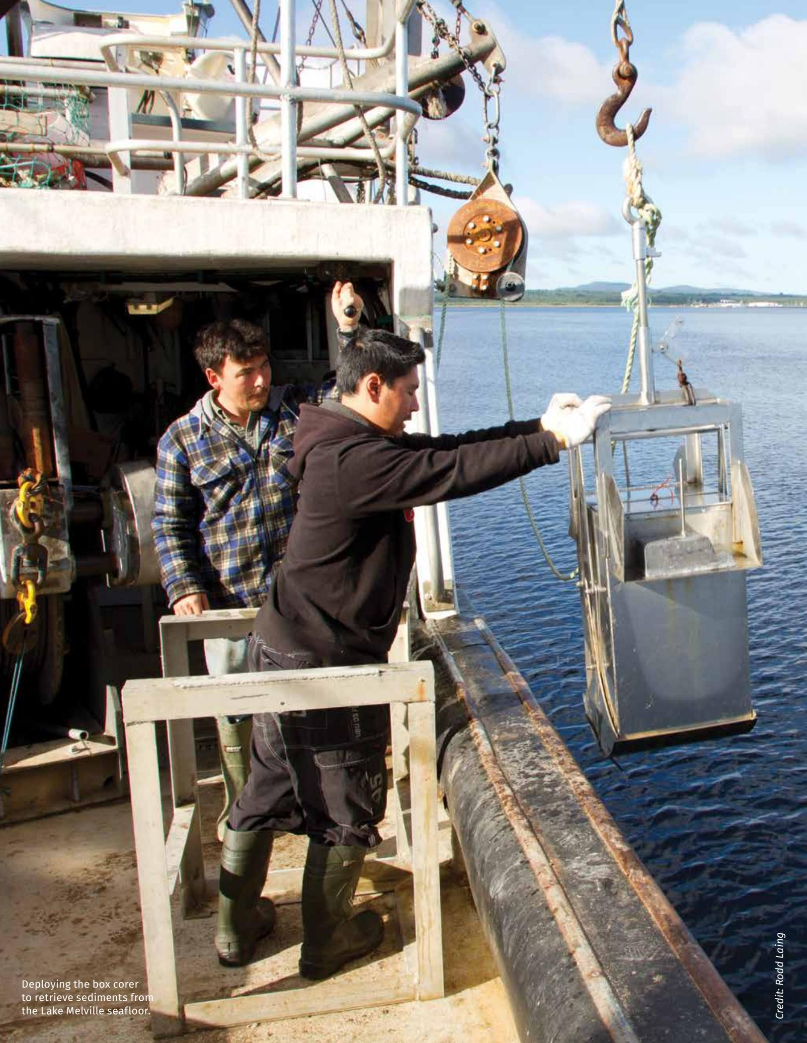
Deploying the box corer to retrieve sediments from the Lake Melville seafloor.
