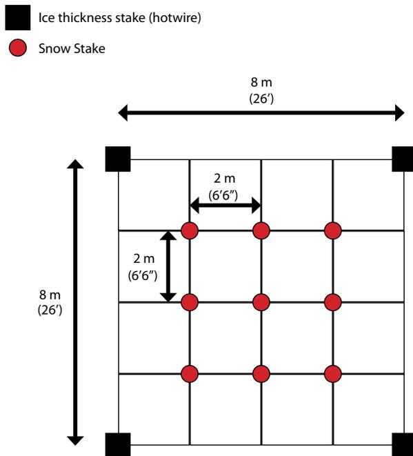
Figure 4.2. Layout of community-based ice monitoring stations. Source: Adapted from Mahoney and Gearheard (2008).
