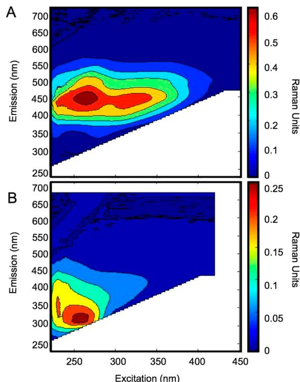
**Figure 2.** Three-dimensional excitation emission matrix (3D-EEM) for Panel (A) Suwannee River reference material obtained from the International Humic Substance Society and Panel (B) marine DOM from Station 6 on the Northwest Atlantic (NWA) continental margin.
